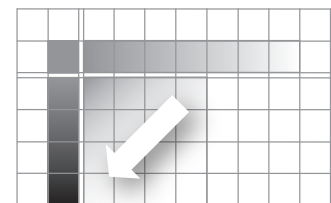
Pixels from the adjacent macroblocks above and to the right are copied diagonally into the intra-coded block
